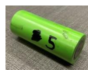
Figure 2. An image of the A123 LFP cell that was both cycled and recycled.
